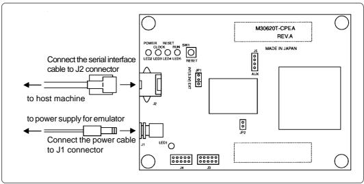
Figure 2.5 Connecting the emulator system
